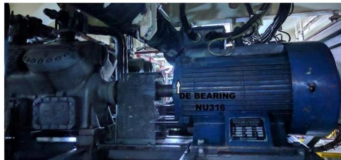
**Figure 3. Motor and compressor of ship's air conditioning system. The location of motor d.e. bearing is highlighted.**
